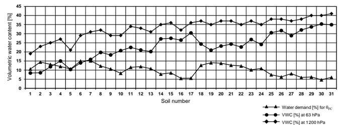
**Figure 3:** Volumetric water contents at simulated stress point (1200 hPa) and at point of simulated field capacity (63 hPa) with the calculated soil-specific water demand.
